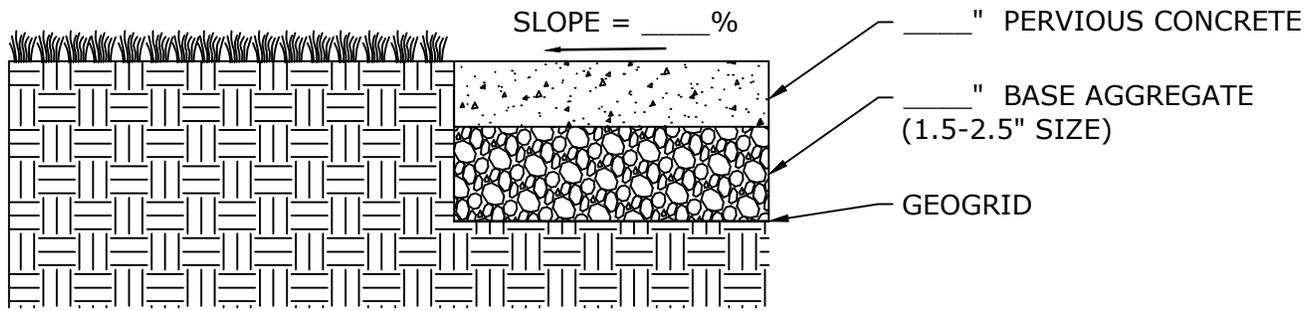
PERVIOUS CONCRETE TYPICAL INSTALLATION
