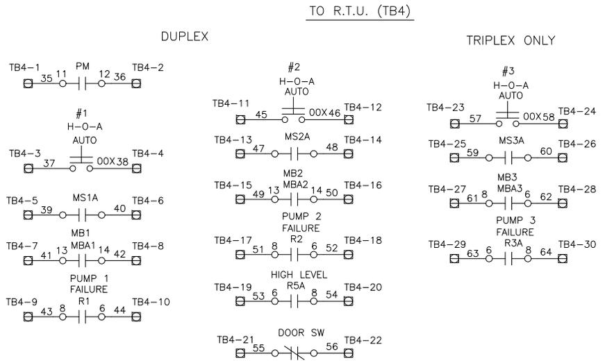
LIFT STATION-SCADA RTU CONTROLWAVE LOOP WIRING
