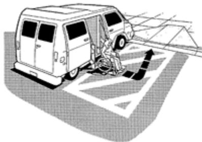
1. 96" min. width access aisle, level (max. slope 1:50 in all directions), located beside the van parking space
